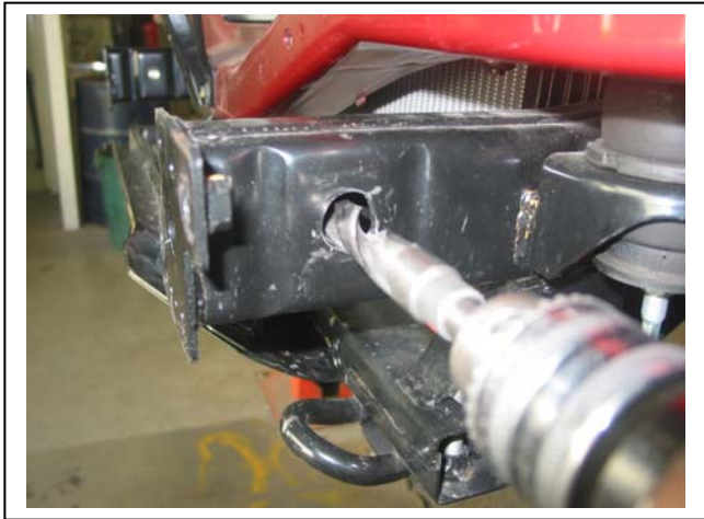
Figure 7: Enlarge front hole in outside of chassis rail.
