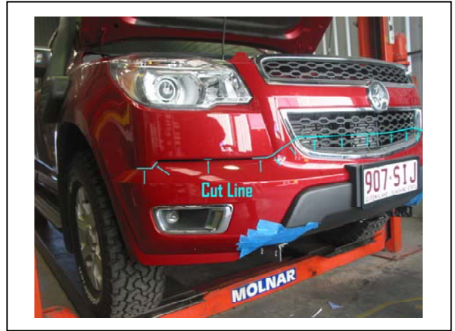
Figure 8: Bumper cut line. Note: cut through grille to allow maximum air flow
