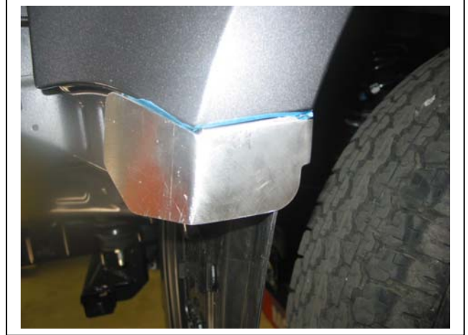
Figure 4: Correct fitment of infill to guard on L/ H side
